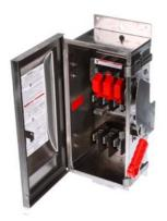
Siemens Low Voltage Circuit Protection Heavy Duty Safety Switches. Type: ENCLOSED, SAFETY SWITCH Std: UL V. Rating: 600V A. Rating: 30 A Wattage: 3W No. Of Poles: 3P F. Rating: 60Hz Action: SINGLE THROW Material: SS Enclosure: TYPE 4X. 2-3 point mounting holes. Insulation: YES O. Cycles: 10000 O. Temperature: (-20F-120F) AMBIENT TEMPERATURE Environmental Conditions: INDUSTRIAL CORROSIVE RESISTANCE
